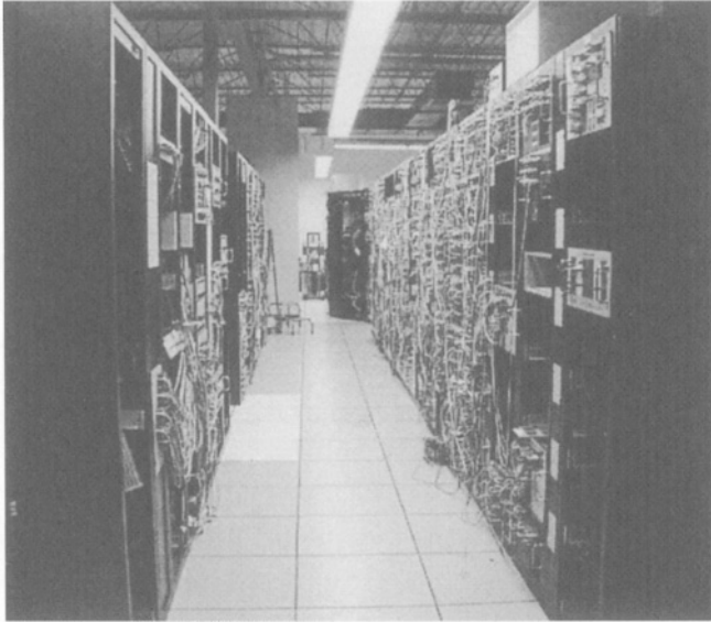
Figure 14-2: Photo shows a row of RLC components connected to model transmission lines
